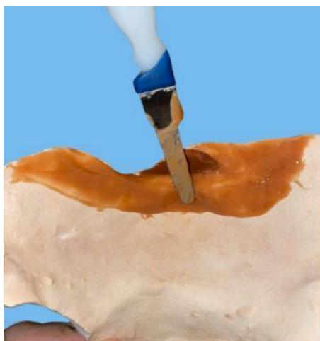
Figure 7 Packing of silicone into the mould
